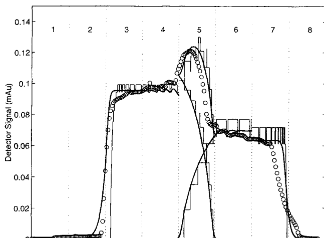
Figure 4a. Experimental results recorded with an on-line detector for \beta_2 = \beta_3 = 1.15 and \beta_1 = \beta_4 = 1.03 .
